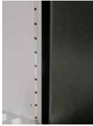
Safety optical barrier (light curtain) in Class 2 (only for MF Plus)
